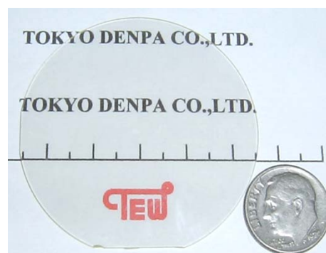
Photograph of 2-inch ZnO substrate
